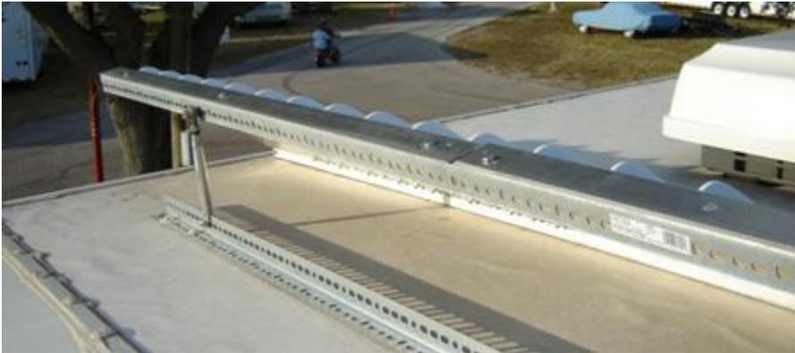
This shows the simple framework we built for the wind deflector and the adjustable struts we used. We lowered the deflector almost 2" from where we started. The less angle the less wind resistance. We used the "bug debris" to get the angle as low as possible.
