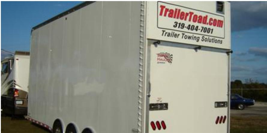
The rear corner of the trailer shows the Air-Tabs located along the rear edge of the trailer. These straighten out the air and prevent the swirling and vacuum normally produced by trailers. The Air-Tabs also eliminated the "side push" we experienced when a semi-tractor/trailer would pass us on the highway.
