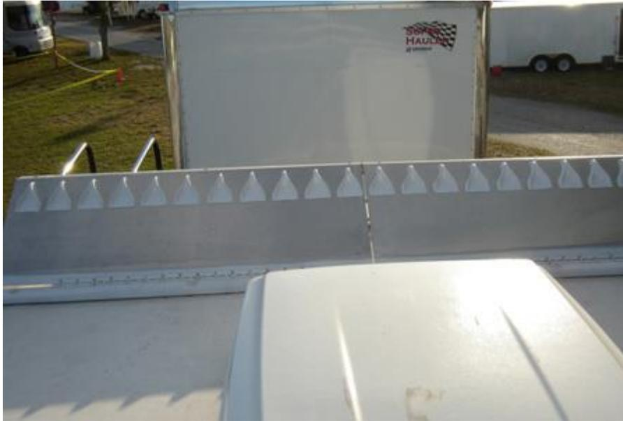
From the front, you can see the wind deflector is just two pieces of flat aluminum that are bolted to a hinge (so it can be raised and lowered). The Air-Tabs on the upper edge assure us the air flow is directed in as straight a line as possible. The Air-Tabs allowed us to run less angle, and thus there is less drag while still getting the air up and over the front of the trailer.
