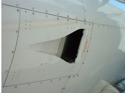
Figure 1: NACA Duct.
