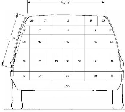
Note: The Yortex Generators are only on part of the sides. Fitting the Yortex Generators across the roof would add another 65% to the perimeter covered by YG's. This would further improve the pressure recovery in the back of the vehicle.
