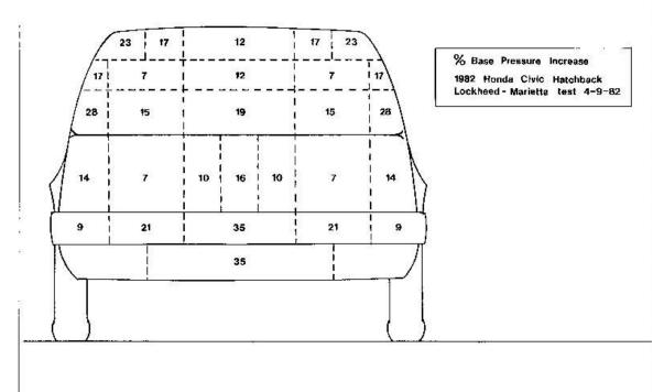
Figure 3; Base Pressure Sensor Schematic. Shows the percentage of base pressure increase for each sensor.
